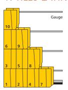
Romane tiles should be laid from the left to right [see tiles numbers beside] Batten size: width 50mm, height 25mm Tiles nailing: on 45° roof pitches [or over], or under very windy conditions, the tiles should be fixed.
