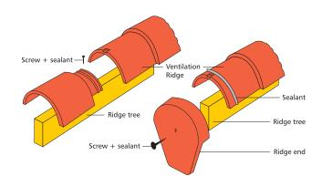
**Ridge end.** They are fixed on the wider part of the ridge [large diameter] to ensure perfect stability. If you happen to finish on a male end, the entire ridge will have to be shifted with a ridge tile cut in half. The ridge should therefore start with the female end of the ridge.
