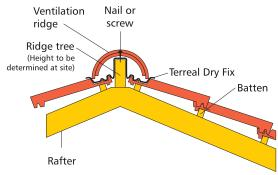
Dry ridge fixing is easy and safe with usage of Terreal Dry Fix adhensive membrane. Benefits: Fast laying-safe from cement leakage and from fungus growth on concrete seals.
