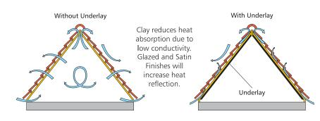
Romane profiles will provide natural ventilation with our large hump allowing better air circulation. In addition, clay, being a poor conductor of heat, will reduce interior temperature by 2-3°C\* as compared to a roof using concrete tiles.
